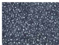
Figure 1a Polarized-light image of a microemulsion made with 5% Olivem®1000 Crystal Skin™ in water
